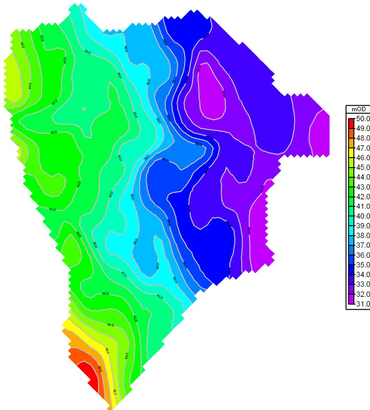
Figure 5: River terrace Deposits thickness with 40 and 37mOD contours from the underlying Tertiary geology topography shown.
