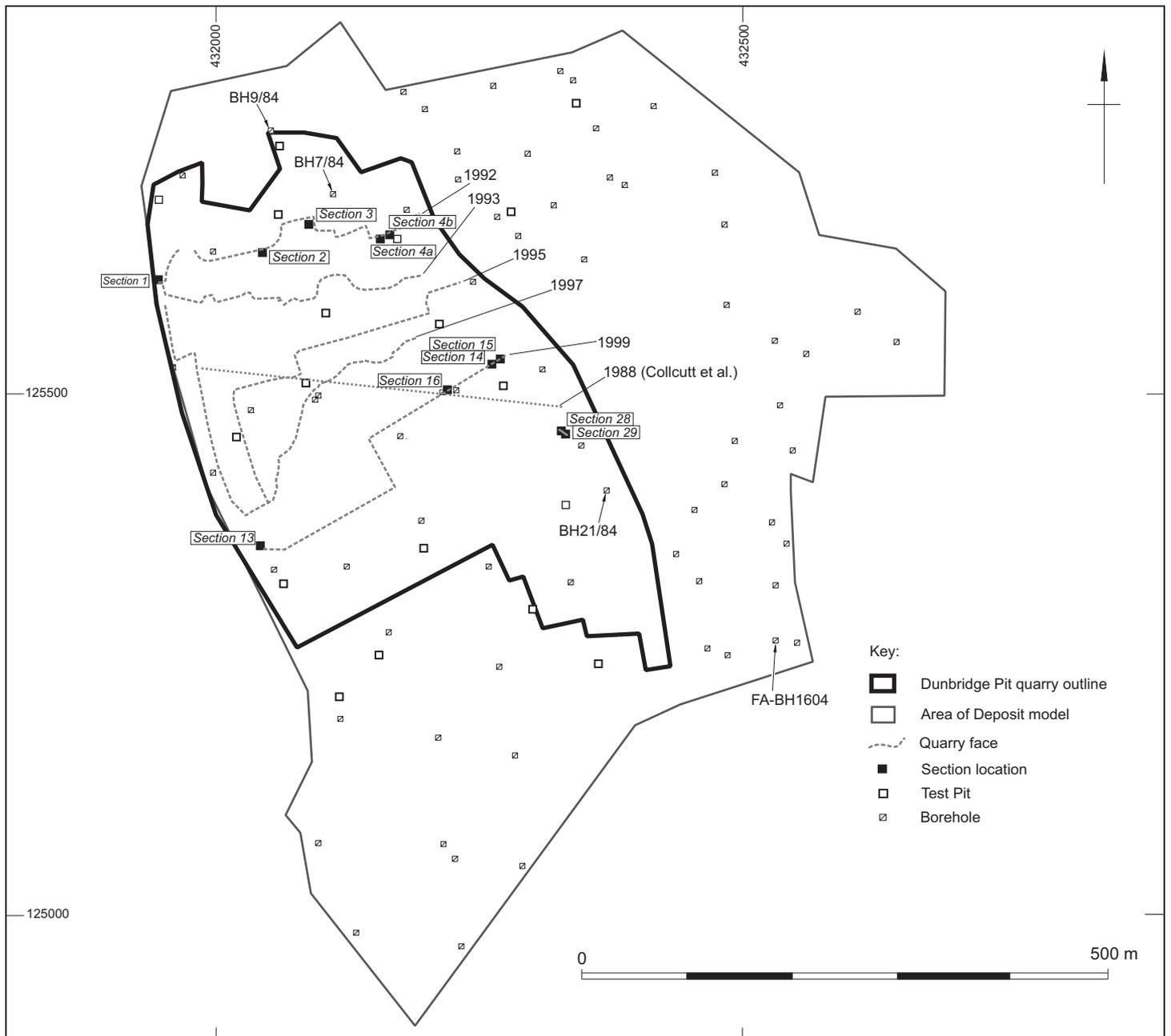
Figure 2: Area of deposit model, showing the distribution and nature of individual sample points (boreholes, test pits and sections).
