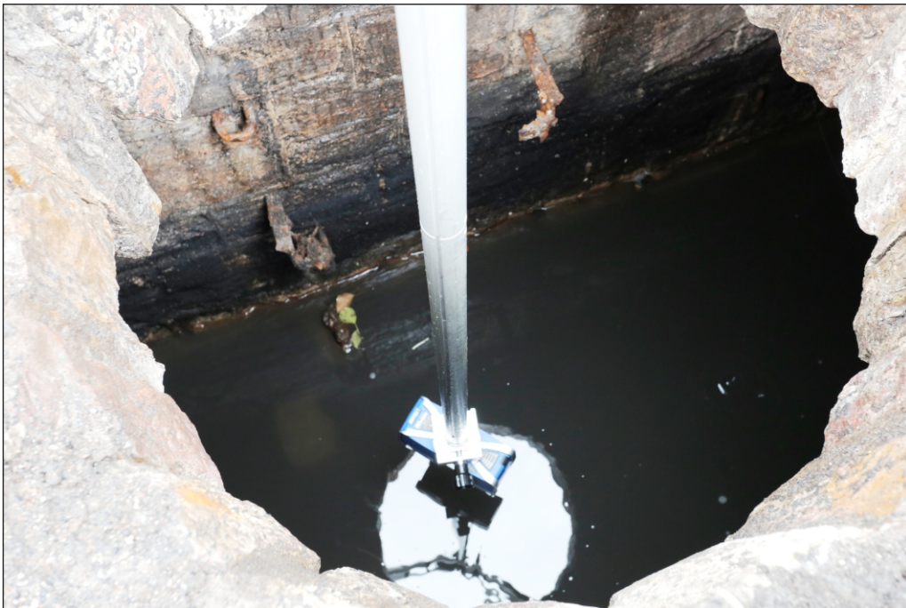
Plate 4: Iron fixings in north wall of east chamber. Laser scanner lowered into chamber
