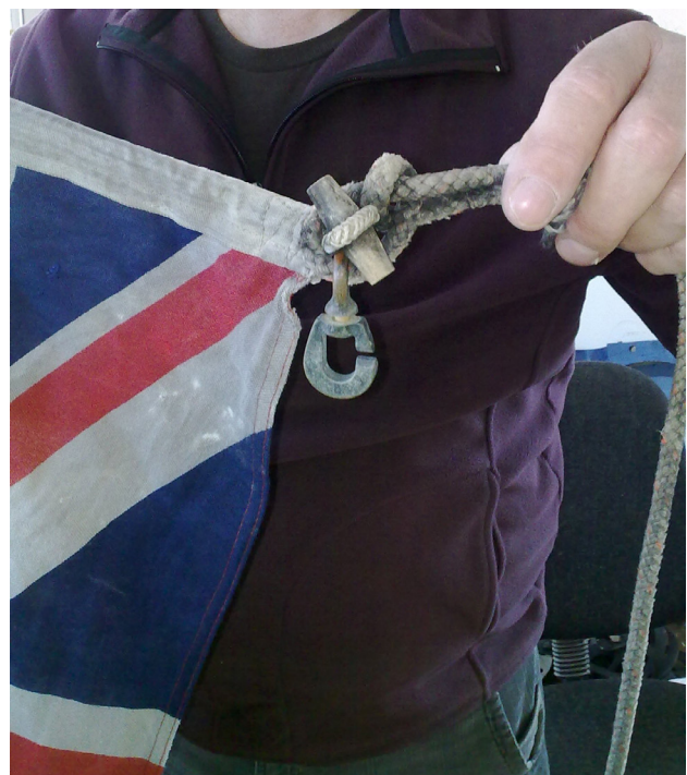
Top: A White Ensign Flag (Tarmac_0978) discovered by Jack Tate; Middle: A Red Ensign Flag (CEMEX_0285) dredged by the Britannia Beaver ; Bottom: the fixing on Red Ensign Flag (CEMEX_0285).
