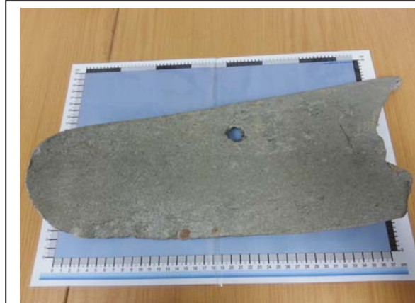
LTM_0515: Propeller blade with bullet hole
