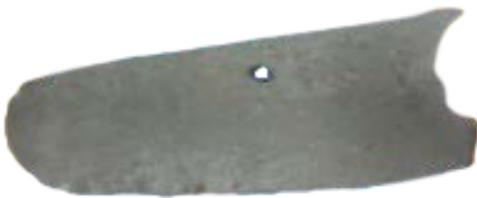
LTM\_0515, a propeller blade with bullet hole
