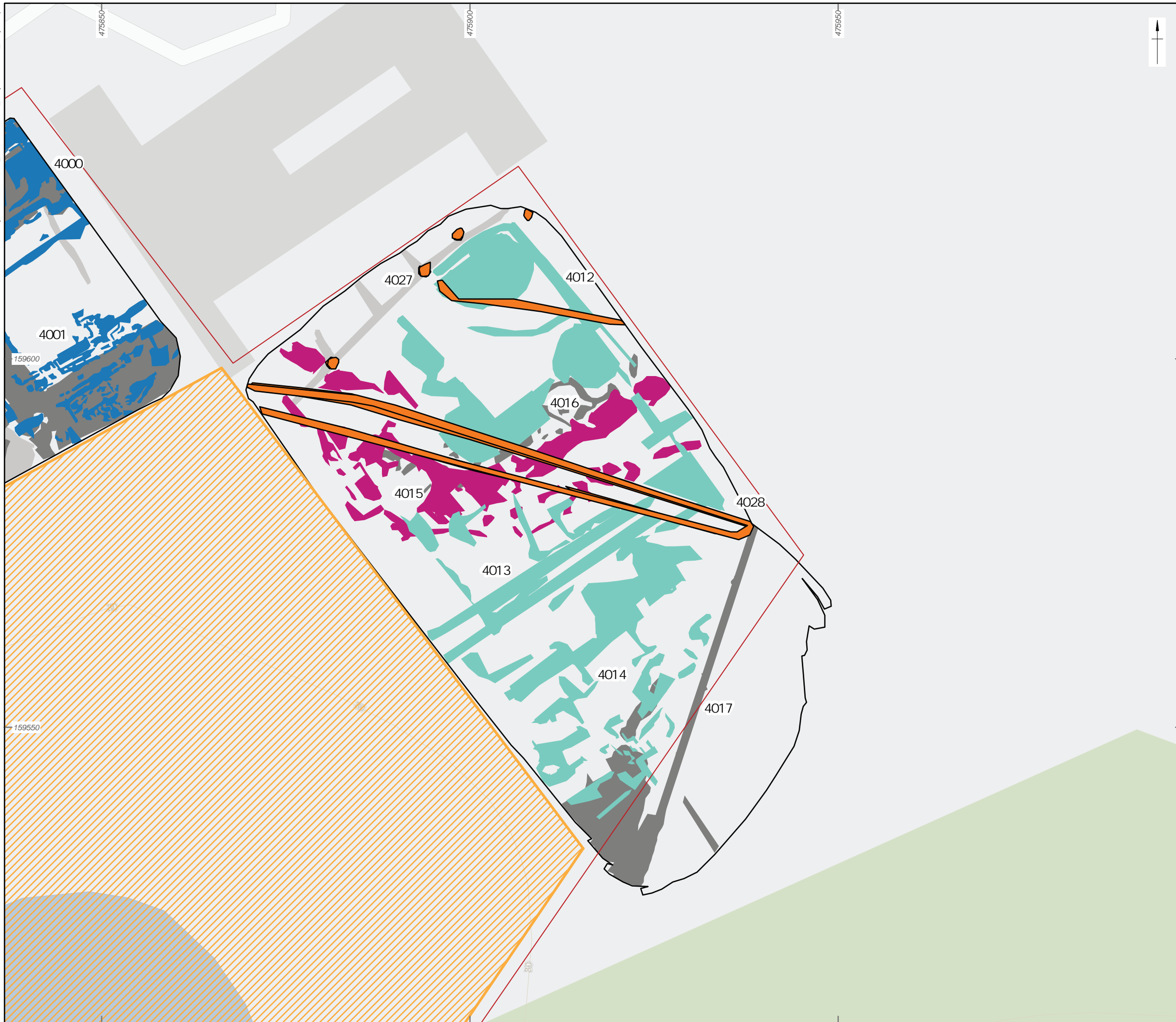
Figure 29: Ground penetrating radar survey results: combined interpretation
