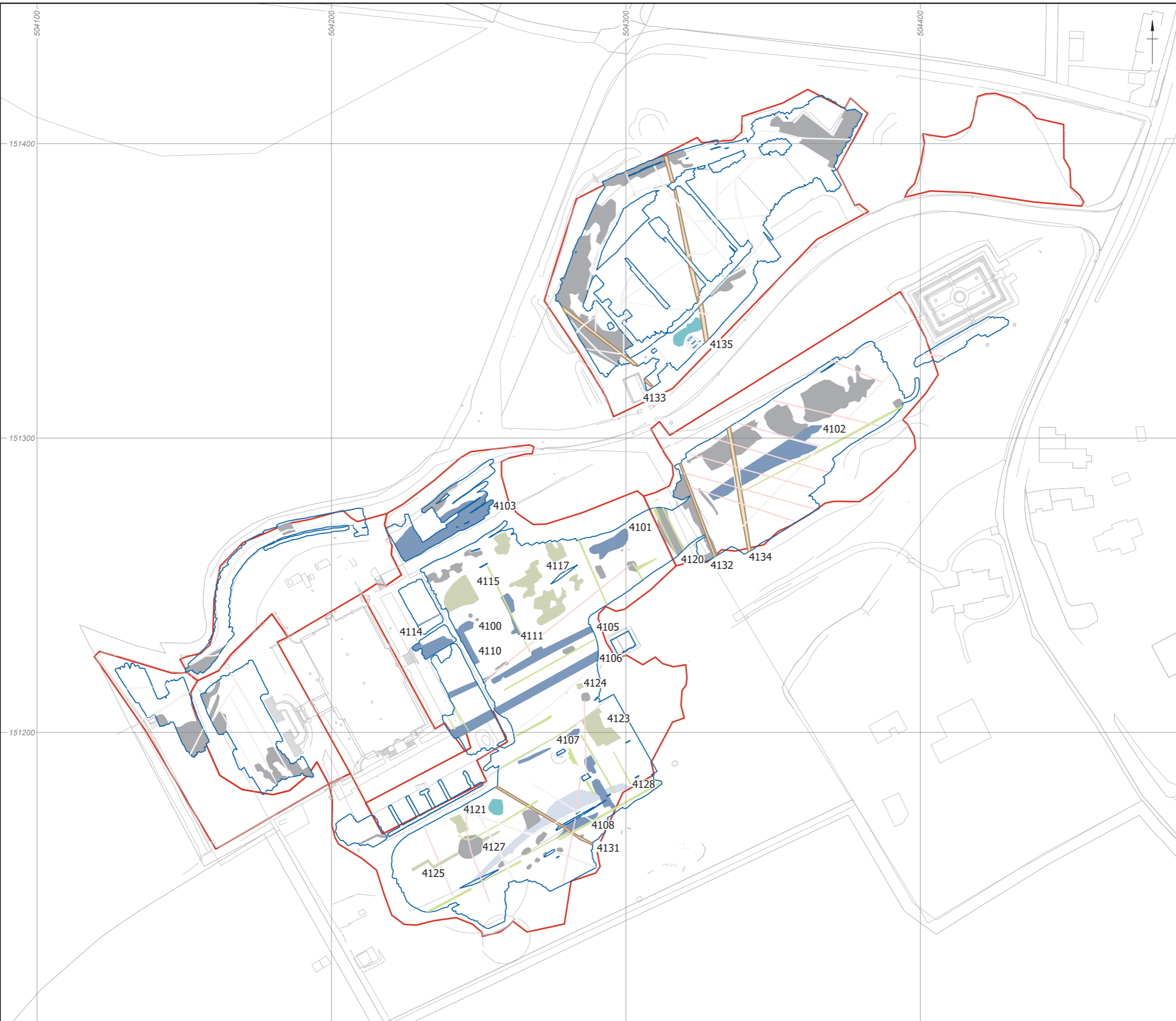
Figure 7: Ground penetrating radar survey results: interpretation Timeslice 5 (0.41 m - 0.51 m)
