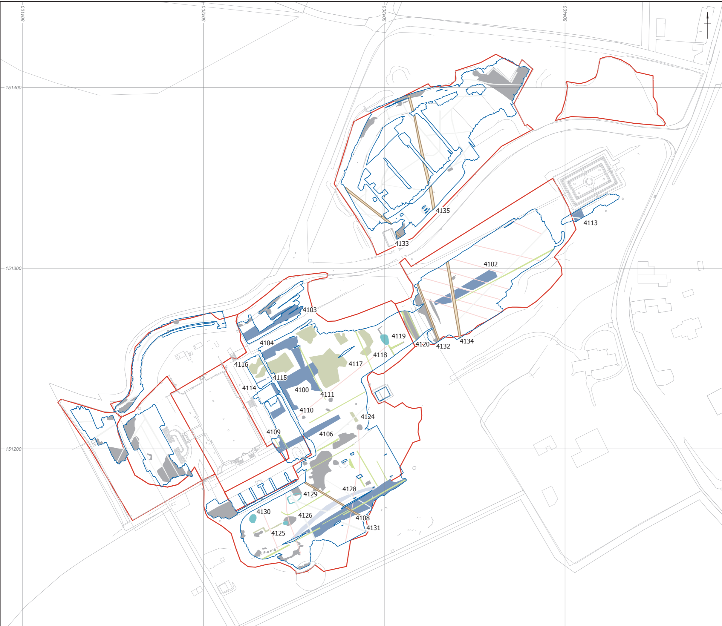
Figure 9: Ground penetrating radar survey results: interpretation Timeslice 7 (0.62 m - 0.72 m)
