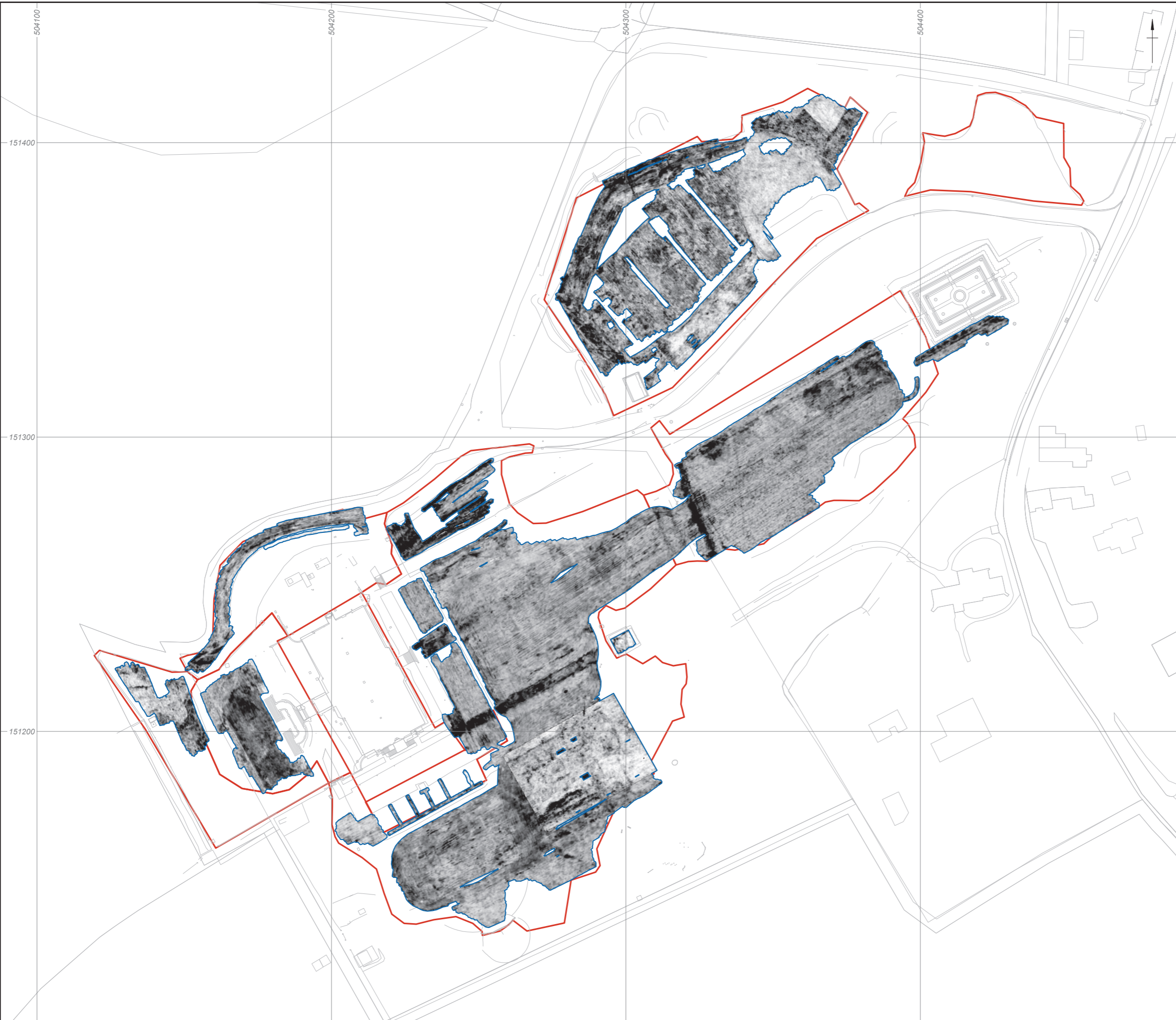
Figure 4: Ground penetrating radar survey results: greyscale plot Timeslice 3 (0.21 m - 0.3 m)
