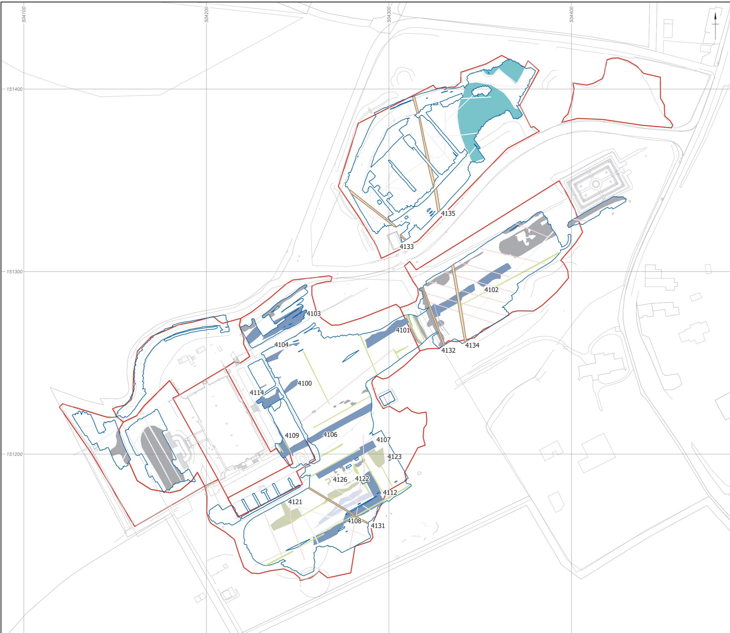
Figure 5: Ground penetrating radar survey results: interpretation Timeslice 3 (0.21 m - 0.3 m)
