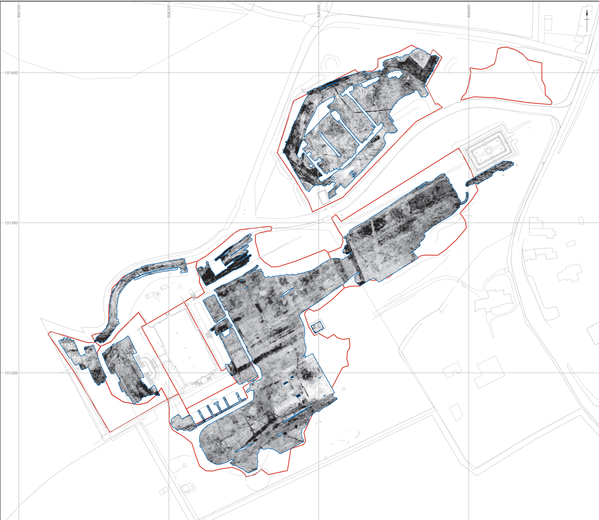
Figure 6: Ground penetrating radar survey results: greyscale plot Timeslice 5 (0.41 m - 0.51 m)
