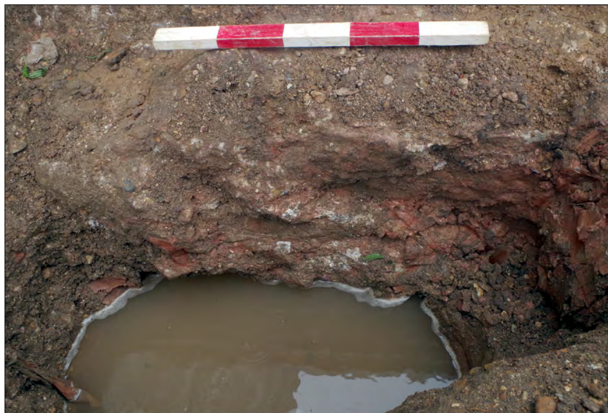
Photo 3) Detail of test pit showing tidal water ingress
