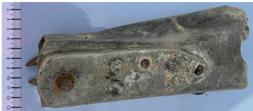
Find d: This is a fragment of aluminium airframe, roughly 200 mm long and 60 mm wide with attached bracket.
