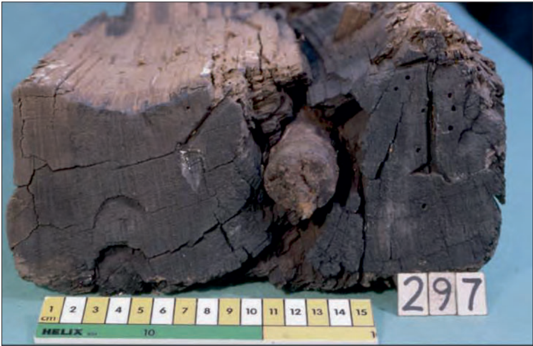
Plate 1: A carved mark on the end of a deck beam denoting the position of the beam in the ship
