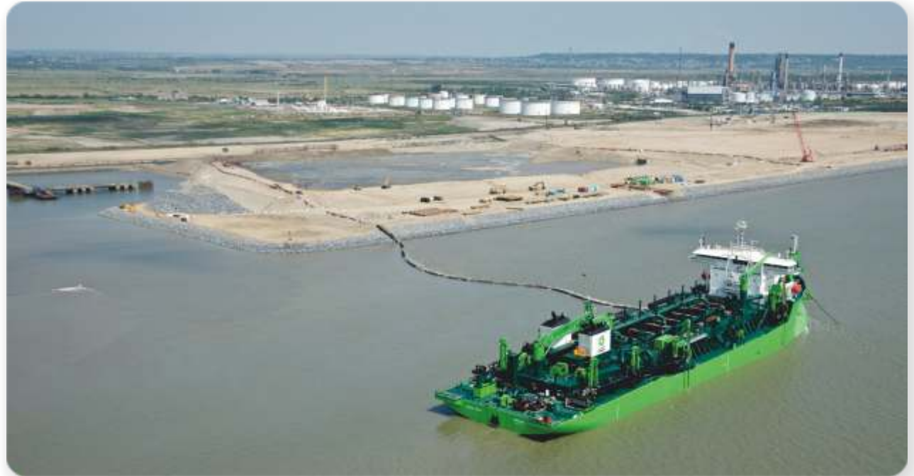
The Congo River unloading dredged material into the reclamation areas during the construction of DP World London Gateway Port
