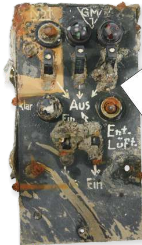
The control unit for the GM-1 boost system
