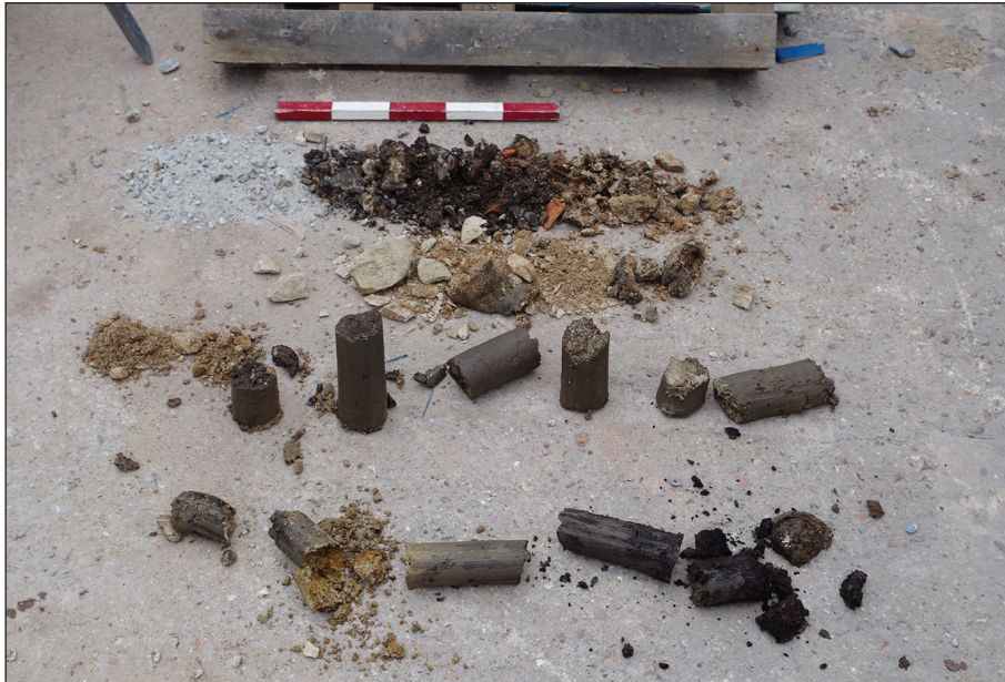
Plate 6: Spoil/core samples from WS01, 0.50 m scale
