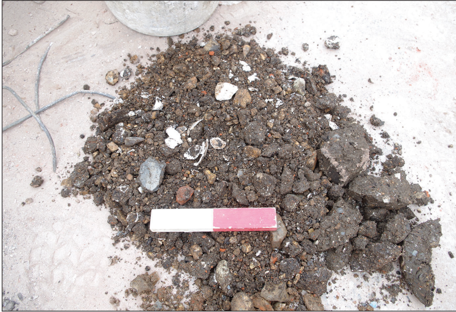
Plate 3: Spoil from cable percussion drilling. Context () – View from East, 0.20 m scale
