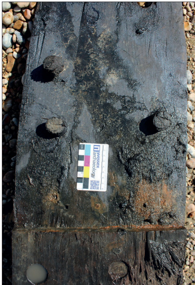
Figure 23: Line of nails at lip of scarf in the outer planking
