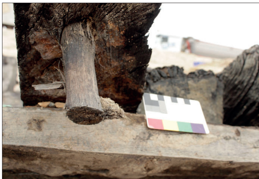
Figure 20: Hemp caulking on treenail
