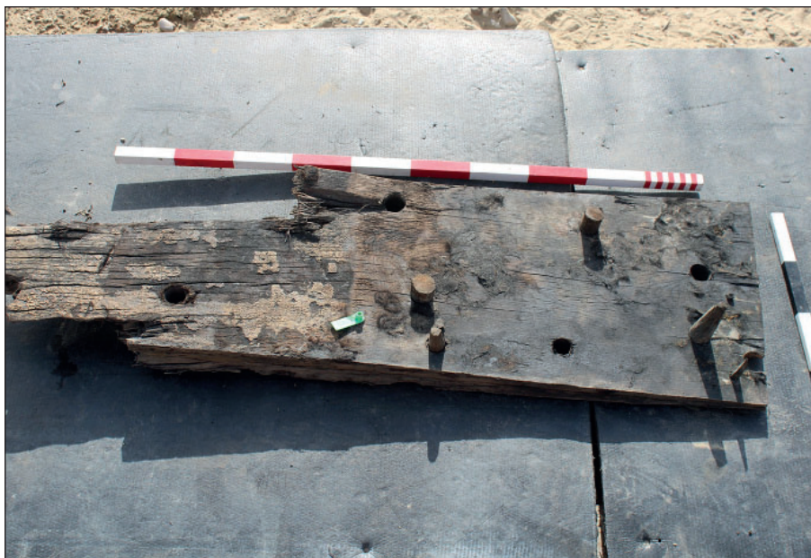
Figure 21: Example of the morphological variety of fasteners at the scarf of plank [098]
