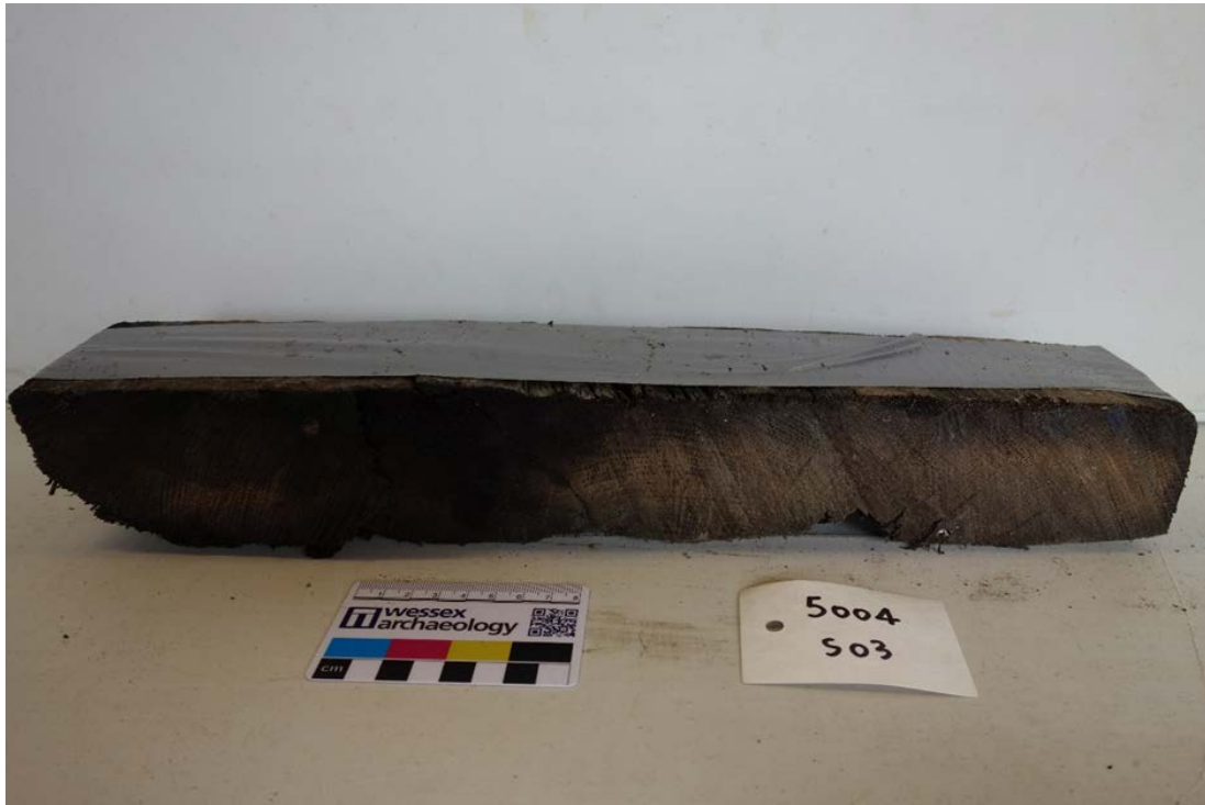
Figure 4a: Oak outer plank sample 079 (vessel section 5004, sample 3) as supplied to the Nottingham Tree-Ring Dating Laboratory. [photograph Wessex Archaeology]
