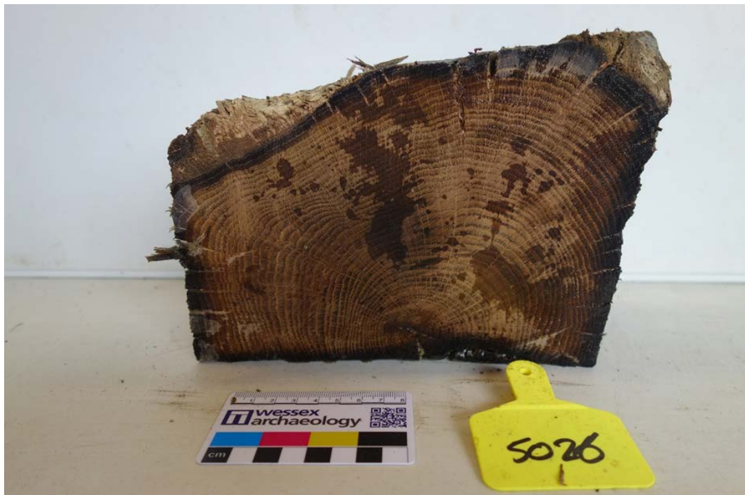
Figure 4d: Oak frame sample 025 (vessel section 5026) as supplied to the Nottingham Tree-Ring Dating Laboratory. [photograph Wessex Archaeology]
