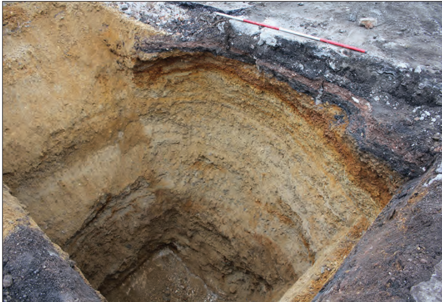
Plate 10: TP25 south east facing section – made ground overlying sandy flint gravel and bedrock chalk
