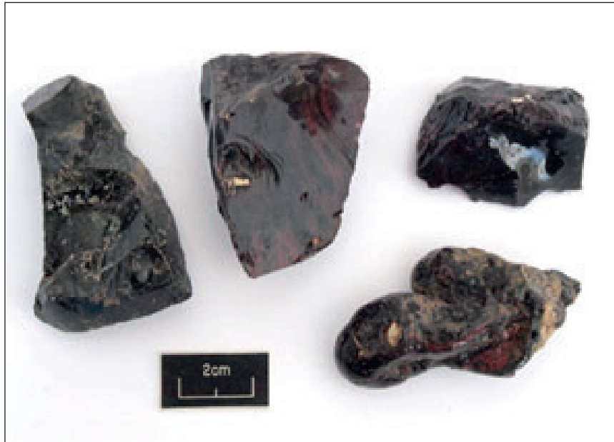
Plate 19: Black Vitreous Waste: showing some reddish colouration from (406)
