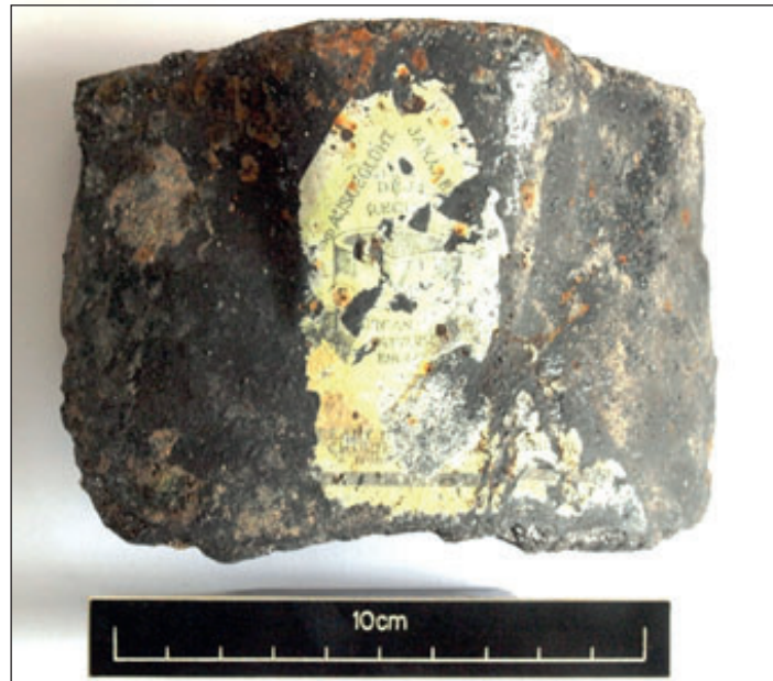
Plate 25: Crucible fragment (unused) from (426). This fragment has a Morgan Crucible Company of Battersea label
