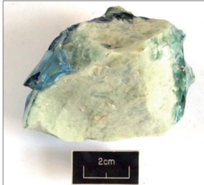
Plate 30: Fragment of devitrified glass waste from (383)
