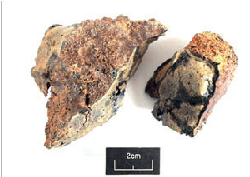
Plate 20: Black Vitreous Waste with abundant crucible fragment inclusions (pot burst?) from (269)
