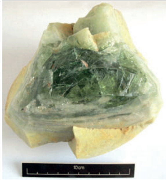
Plate 31: Devitrified glass waste from (426)
