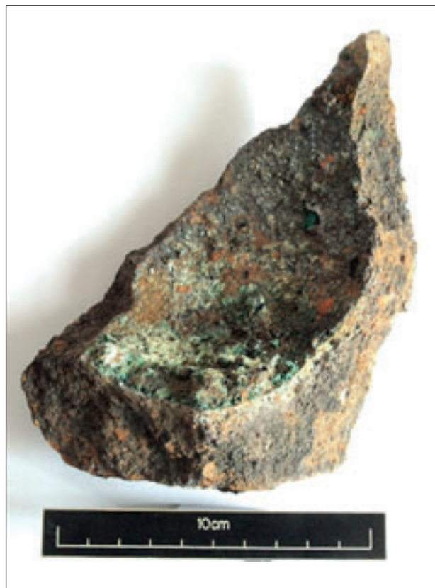
Plate 24: Crucible fragment from (426). The presence of green copper corrosion products suggests that this crucible was used to melt copper alloys rather than glass.
