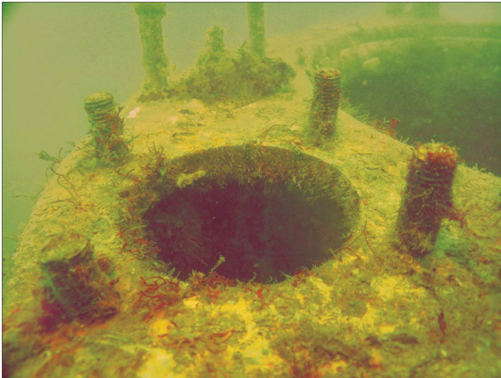
Plate 3: Brass bolts for missing periscope mount
