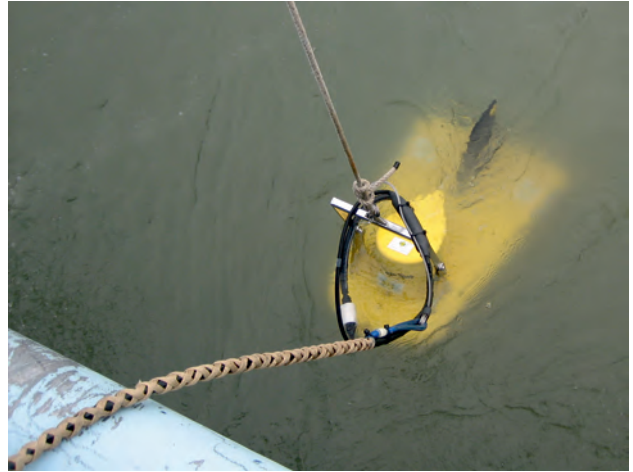
Plate 3.2 Deployment of chirp sub-bottom profiler system
