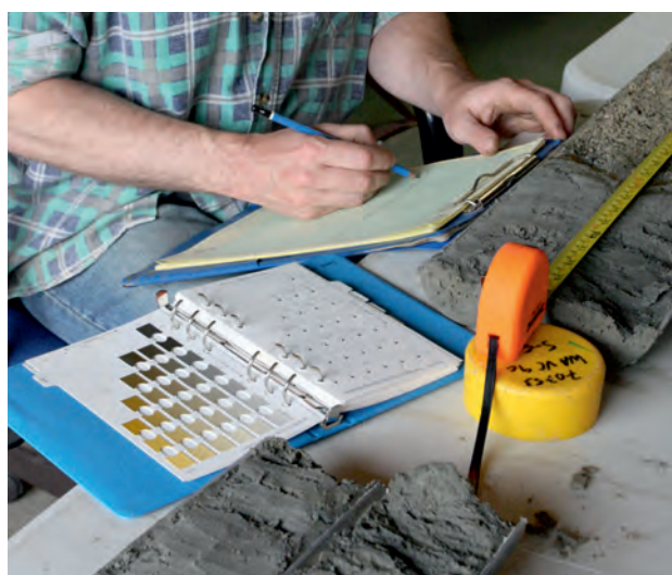
Plate 3.5 Geoarchaeological recording of a vibrocore
