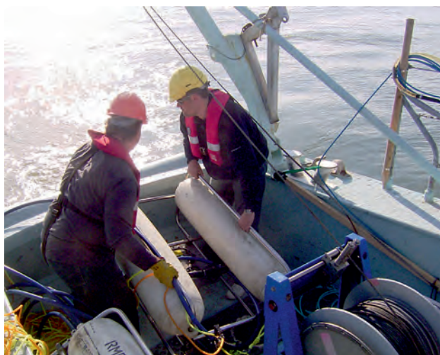
Plate 3.1 Deployment of surface-tow boomer sub-bottom profiler system
