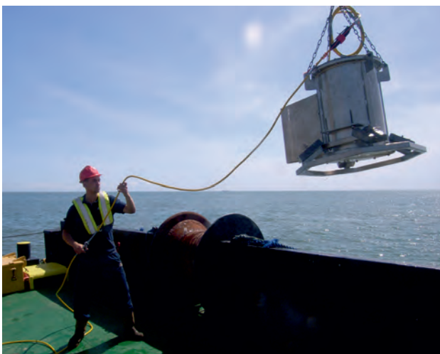
Plate 5.3 Deployment of the ELVIS drop-down camera
