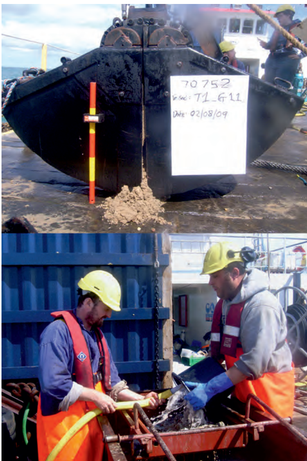
Plate 5.5 Recovery of the 280 litre hydraulic clamshell grab sample and on board processing of the sample through a 10 mm sieve
