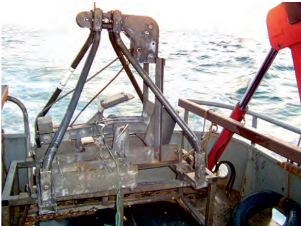
Plate 5.1 The Hamon grab deployed from the vessel to sample typically 10–15 litres of seabed sediment
