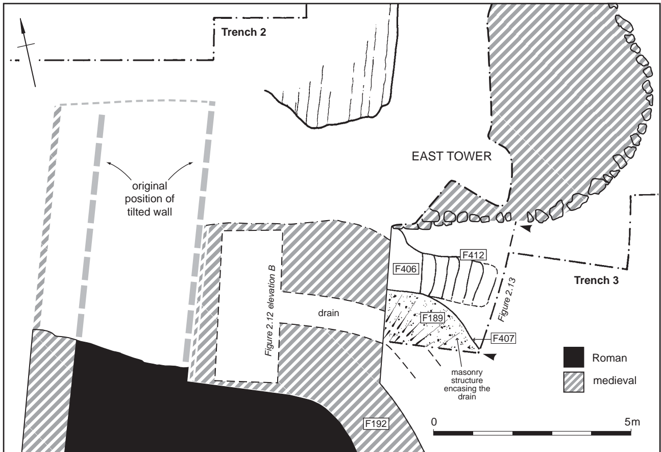
Figure 2.11 Plan of garderobe chamber inserted between the Keep's East and South East Towers in Phase 9 (see Figure 1.3 for location). Note that the fragment of tilted Roman fort wall, with a medieval inner facing, has been restored to its original position (see Figure 2.12 for its actual current position)
