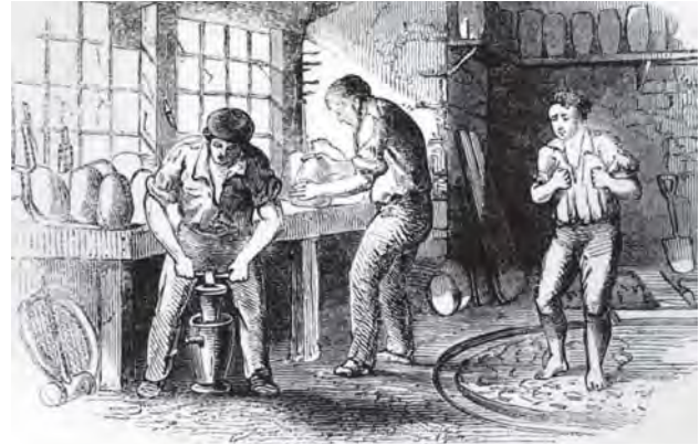
Figure 9 Making crucibles for melting, treading the clay (Sheffield Local Studies Library Picture Sheffield s10816)
