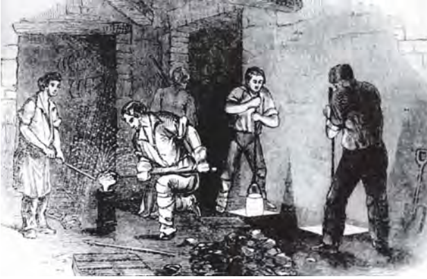
Figure 8 Casting ingots, drawing the crucibles (Sheffield Local Studies Library Picture Sheffield s10815)
