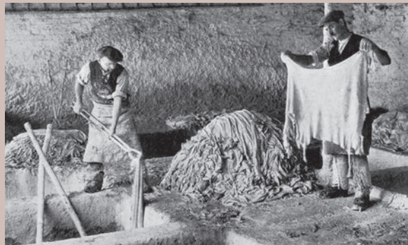
Plate 4.26 Soaking sheepskins in liming pits to arrest putrefaction and remove fat. Image of the Homewell Parchment Works, Havant, published in The Sphere, 28 September 1928, 208 © Mary Evans Picture Library
