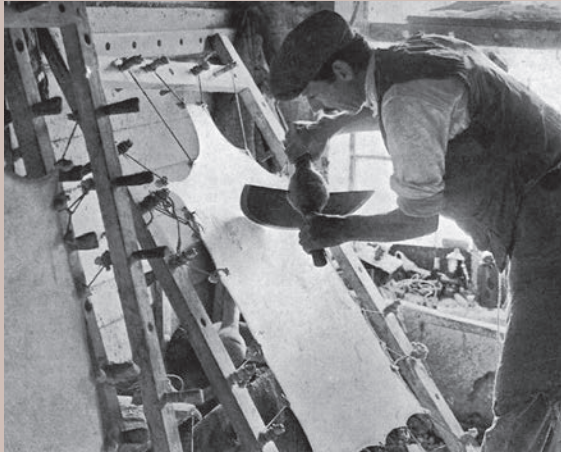
Plate 4.27 Worked sheepskins fixed to a frame then scraped with a half-moon knife to remove excess flesh, dirt and slime after soaking in liming pits. Image of the Homewell Parchment Works, Havant, published in The Sphere, 28 September 1928, 208 © Mary Evans Picture Library
