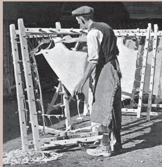
Plate 4.28 Finished parchment being cut from a frame. Image of the Homewell Parchment Works, Havant, published in The Sphere, 28 September 1928, 208 © Mary Evans Picture Library
