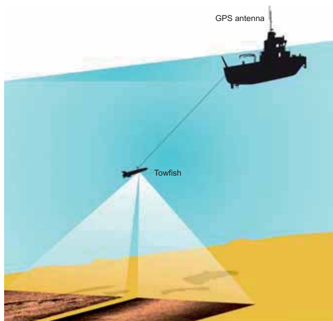
Figure 11: Sidescan sonar towfish
