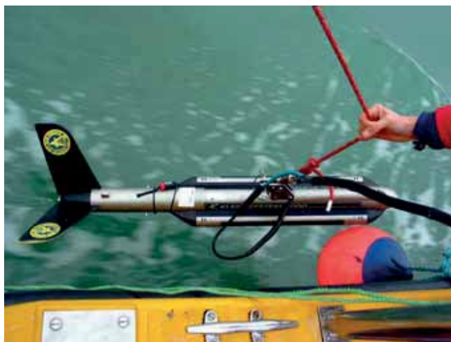
Figure 10: Deployment of a sidescan sonar
