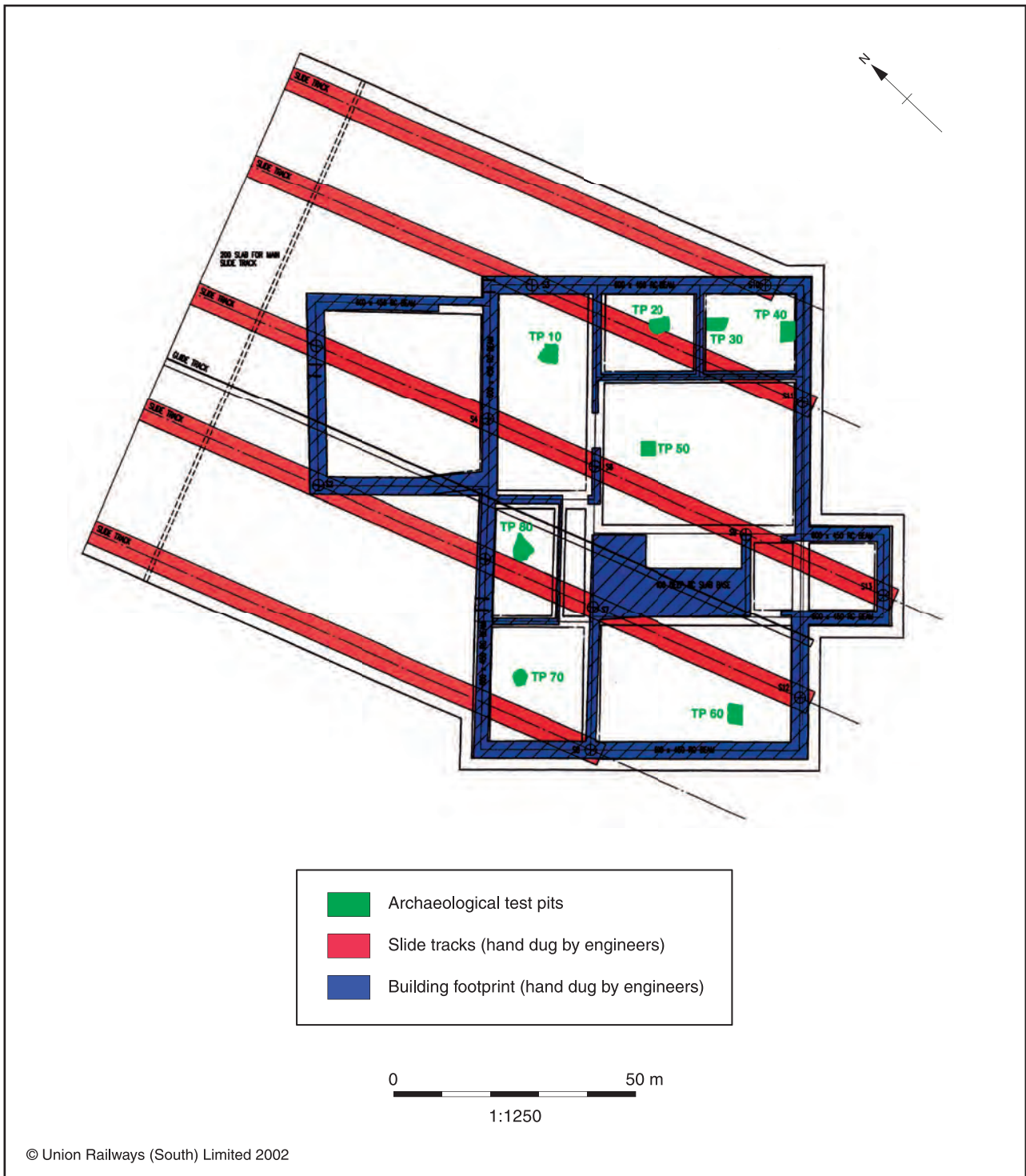
Figure 7.28 Bridge House: ground plan showing excavated areas
