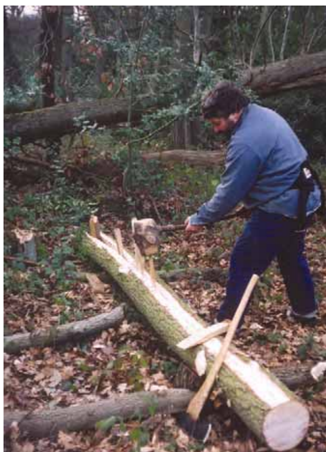
Plate 6.10 Splitting (cleaving) an oak log with wedges to replicate half log piles used in the mill
