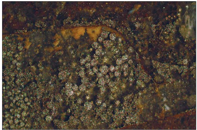
Fig 21: As Fig 19, under oblique incident light (OIL); note typical brassy colour of pyrite.
