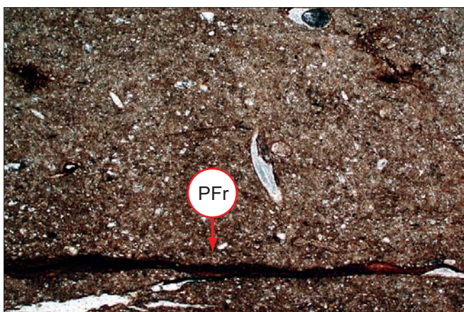
Fig 34: Photomicrograph of M2 (19549) (see Fig 16); dumped layers of silty clay sediment that include long horizontally oriented plant fragment (PFR). PPL, frame width is ~4.6 mm.
