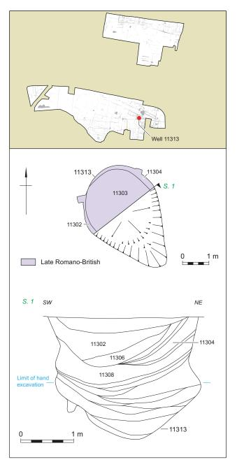
Figure 4.12 Well 11313: plan and section
