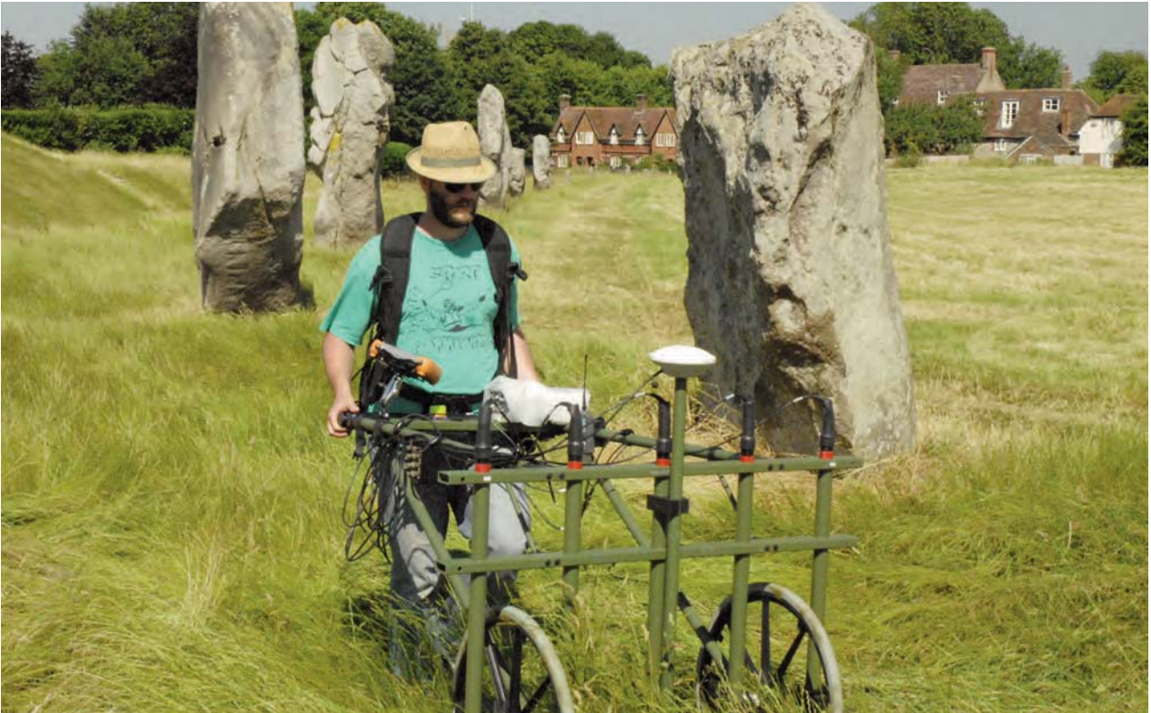
Multi-sensor hand-cart gradiometer at Avebury, July 2013 (Photography by Timothy Darvill © Bournemouth University and Deutsches Archäologisches Institut)
