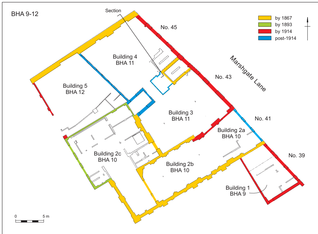
Figure 6.19: Phased ground floor plan of BHA 9–12
