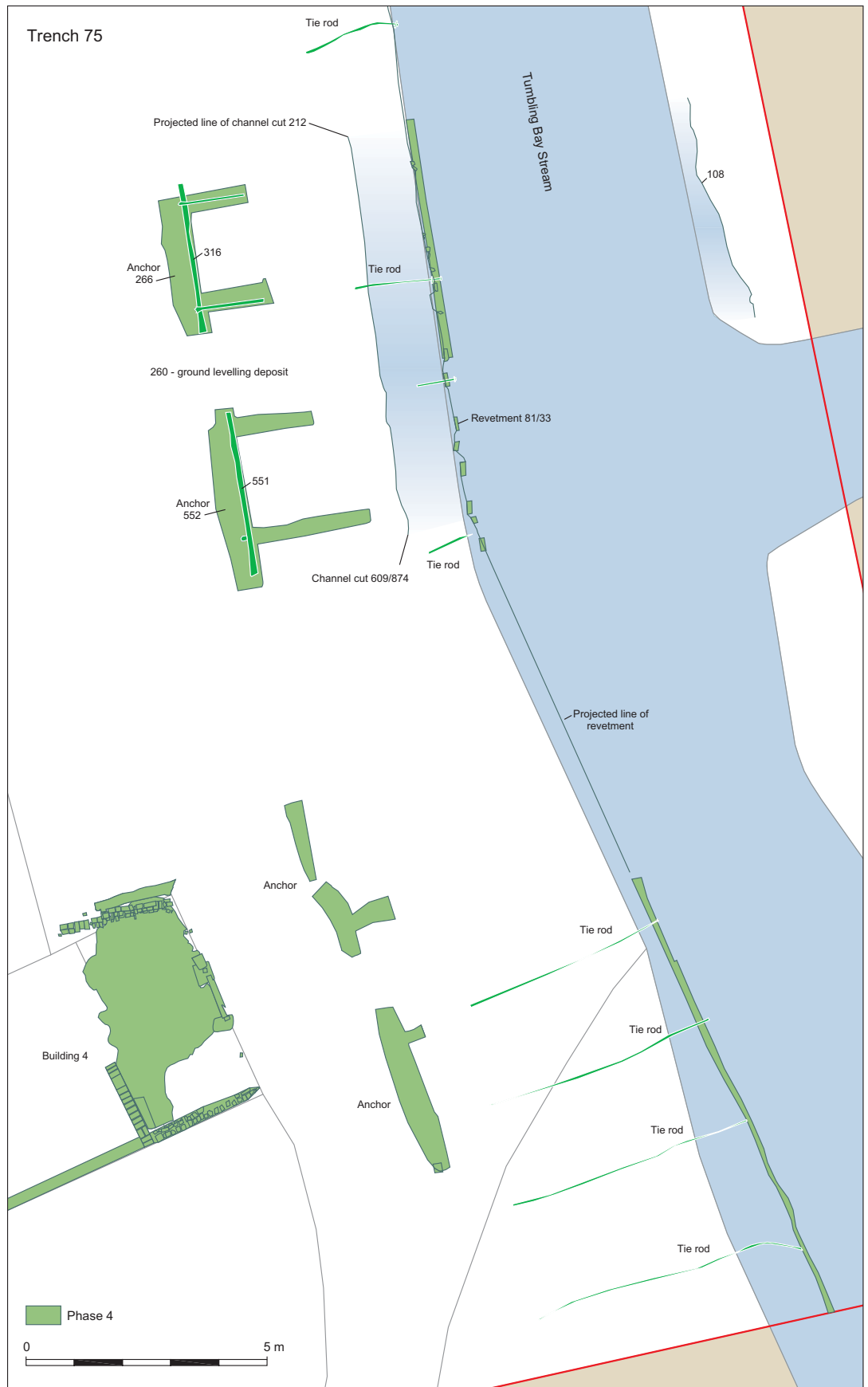
Figure 6.8: Trench 75: Phase 4 revetment of Tumbling Bay Stream with tie rods and anchors
