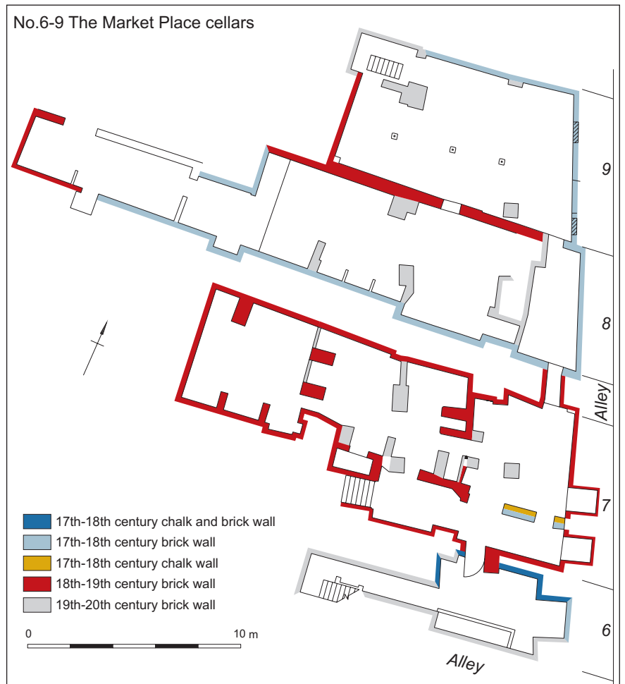
Figure 107: Plan of 17th century and earlier cellar remains beneath the Market Place frontage at Charter Quay.
