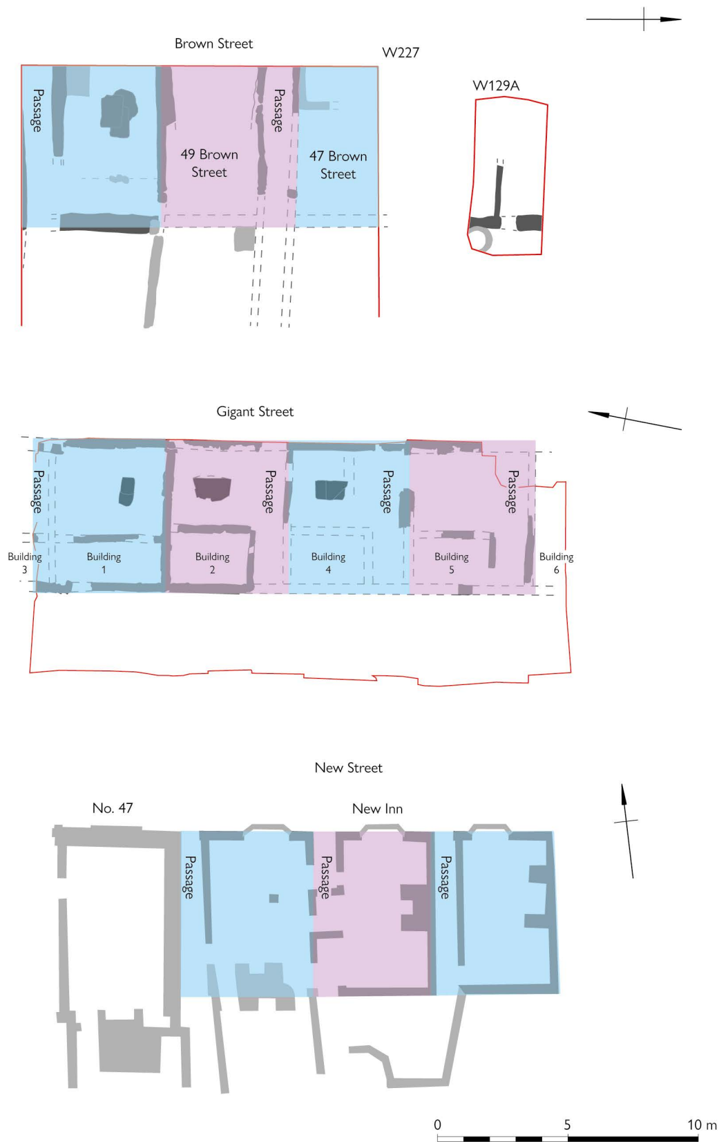
Figure 4.9 Ground plans of Nos 47–51 Brown Street, Anchor Brewery, Gigant Street and New Inn, interpreted as individual cottages
