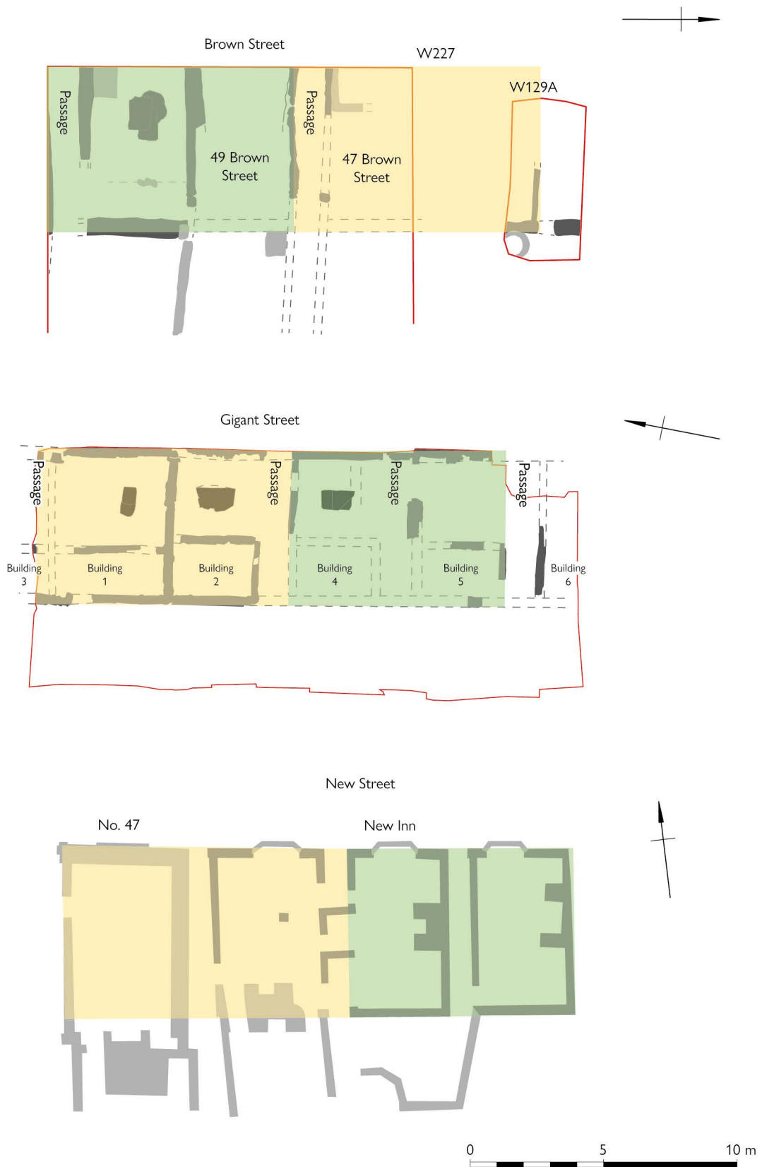
Figure 4.10 Ground plans of Nos 47–51 Brown Street, Anchor Brewery, Gigant Street and New Inn, interpreted as paired units to include an open hall and adjoining chamber
