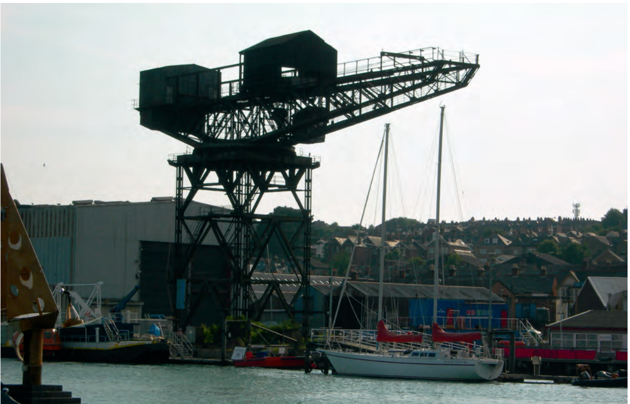
Plate 17.11 Hammerhead Ship Crane at Cowes on the Isle of Wight, copyright Isle of Wight Museum
