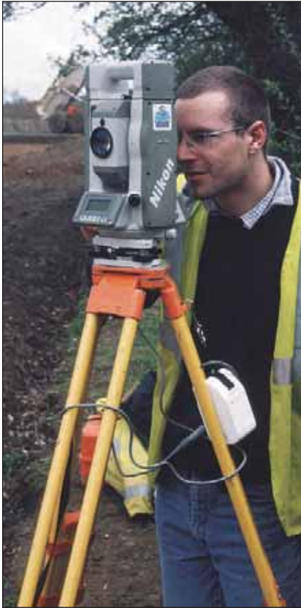
Plate 1.2: Digital surveying using a Total Station EDM
