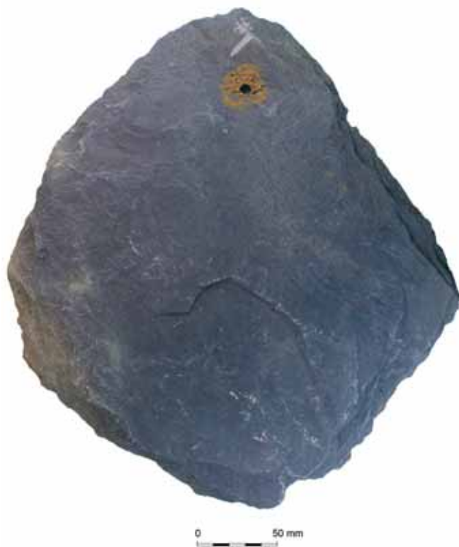
Fig. 4.87 Diamond-shaped stone roof slate
