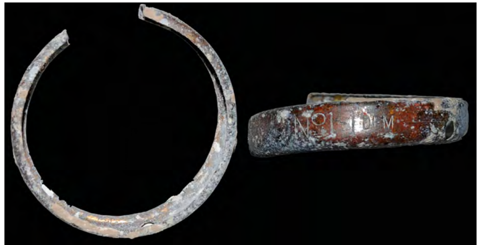
Figure 7.18 Fuze collar marked 'No 1 - 1', indicating the type, and 'DFM', indicating the manufacturer
